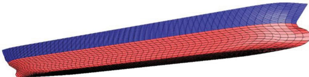
**Figure 3.** Panel model on ship hull for WASIM calculations (full load, bulbous bow), red part is below calm water surface, blue part is above water surface. Blue part is only used for nonlinear WASIM simulations.
